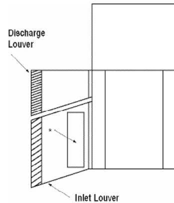
\* Access panel for condenser coil cleaning
