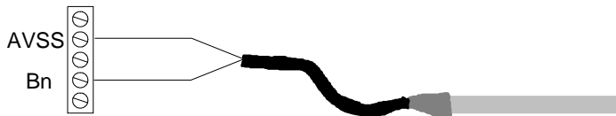
Figure 16 – Temperature Sensor Termination References
